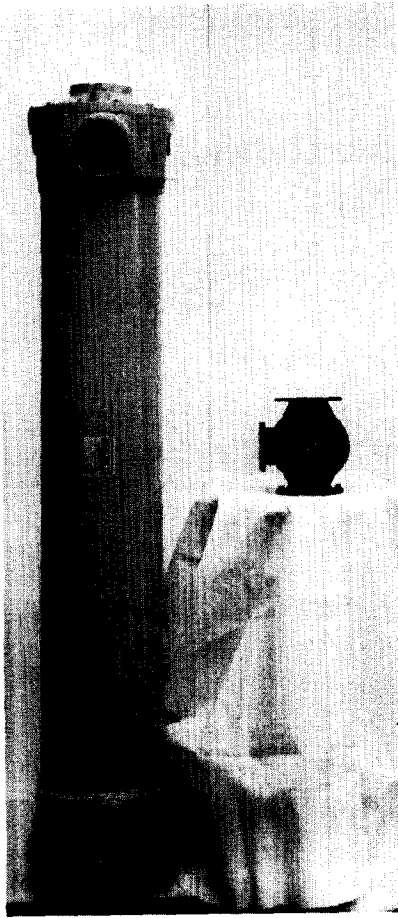
FIG. 1. Comparison of compact heat exchanger (right) used as a boiler and a conventional tube-and-shell condenser (left) of equal heat duties.
